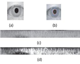
Fig.4: (a) Original image; (b) localized iris; (c) normalized iris; And (d) enhanced iris.
